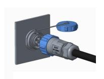
7. Align with the white dot on connectors, then locking the plug and socket with torque of 0.8-1.2N.m
