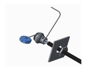
4. Tighten the contact screw via Allen key.
