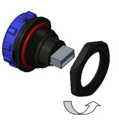
3. Tighten the rear-nut according to torque of 1-1.1N.m
