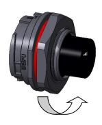
2. Put the socket into the panel. (max panel thickness:3mm)
