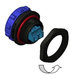
3. Tighten the rear-nut according to torque of 1-1.1N.m
