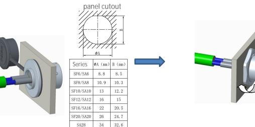
(4) Tighten the socket body and panel closely
