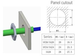
③ Put the stripped cable through the locknut and panel based on above panel cutout size (panel thickness: 4.5max)
