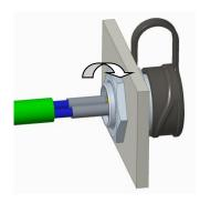
⑤ Tighten the locknut according to torque of 1.0-1.1N.m
