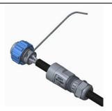
4. Tighten the contact screw via Allen key.
