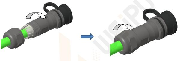
Tighten the backshell and the main part clockwise according to torque of 0.9-1.0N.m
