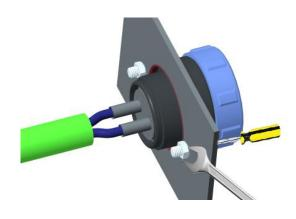
**Caution**: Do NOT apply sealants on plastic connector housings, which may lead to connector breakage.
