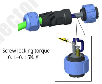
5. Tighten the compression nut and backshell clockwise according to the below torque
