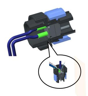
2. Put the stripped cable through all parts
