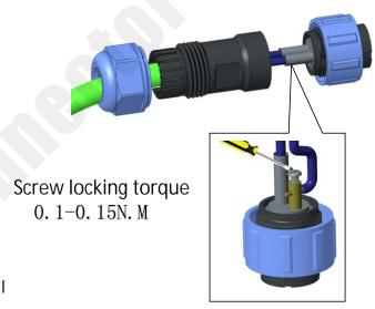
4. Tighten the backshell and the main part clockwise according to the below torque
