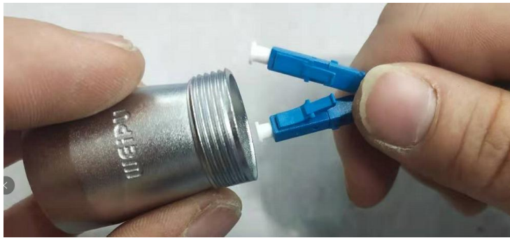
Put the WY24 series shell through the LC pins (Fig. ⑥)
