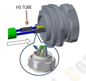
Unscrew the cap and locknut after soldering the wire, then install the socket on the panel closely.
