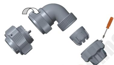
3. Put the stripped cable through all the parts
