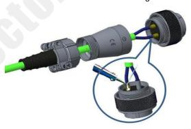
4. Tighten the backshell according to below torque.
