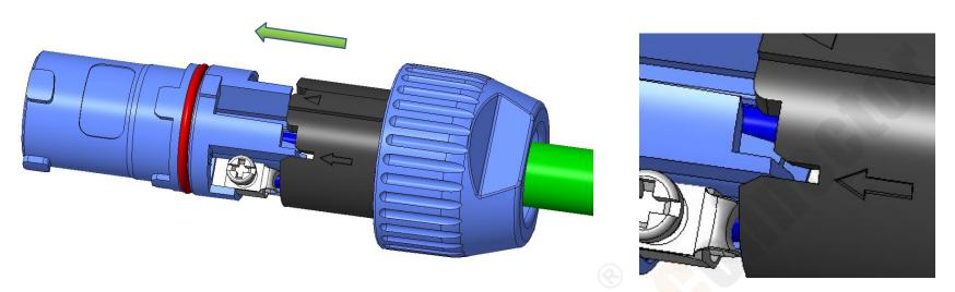
4. Align the two triangle marks as show in below picture, push in axially to the end, tighten the compression nut with torque of 0.9-1.2Nm
