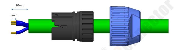
2. Put the wire into contacts and tighten the wire with screw ( Torque 0.15-0.2Nm ) ;
