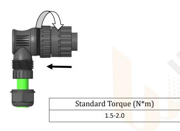
5. Tighten the compression nut according to the torque.
