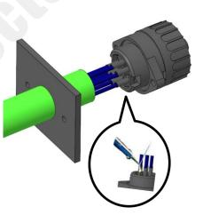
4. Tighten the screws to fix the socket.
