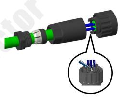
4. Tighten the backshell according to the torque.
