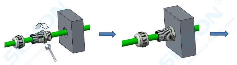
④ Tighten the main part on the panel by using a wrench. Refer to the torque listed in below table.
