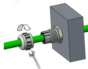
**©**Tighten the compression nut and the main part by using a wrench.
