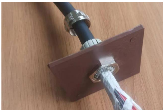
7 ) Locknut assembling finished
